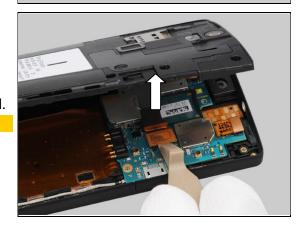
Unsnap the BtB connector by using the Front Opening Tool. *No conductive tools should be used!*
