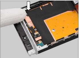
Apply 12 Ncm +/-1Ncm torque when tightening the two Screw Len:3.5 Diam:1.4 with Bits (JCIS No 0).
