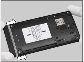
Apply 10 Ncm torque when tightening the three screws
