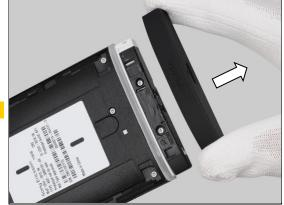
Remove the Cover Bottom with your fingers. Scrap! Not to be reused! Remove the three screws Len:3.5 Diam:1.4M by Bits(JCIS No 0).
