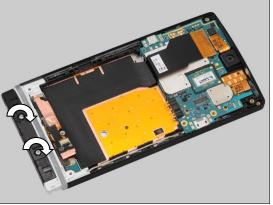
Apply 10 Ncm torque when tightening the two Screw Len:6.0 Diam:1.4 with Bits (JCIS No 0).
