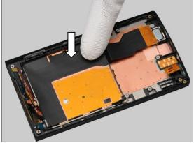
Secure the FPC Main Assy in the correct position, by sliding it under LCD FPC slot as shown in picture!
